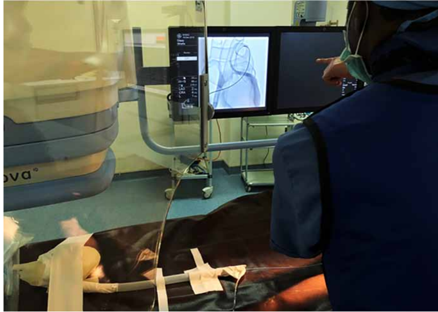
Fig. 4: The 3D printed heart model is fixated on the patient table for imaging via the C-arm(s) of the X-ray machine. Due to the use of radiopaque printing material the contours of the model are visible for the cardiologists in the X-ray images on the transmission screen.
